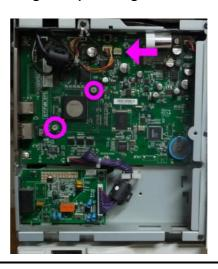
7. Attach the new fan back to the two spacers that remained on the circuit board using the two remaining screws.
