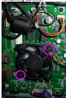
8. Due to variation in production on behalf of Lexmark, it is not possible to equip the replacement-fan with a plug fitting all lots of this printer model. In particular cases it might be necessary to make some little adjustments.
